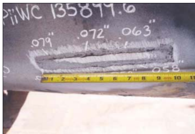
These photos show corrosion beneath wood pieces attached to the transmission pipeline by wire as casing spacers. The right photograph is a detail of the same damage shown in the left (photo from Kinder Morgan; Fig. 3).
